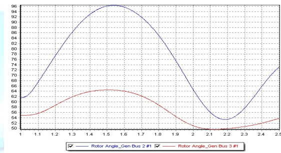
Fig 6: Rotor angle response at a clearing time of 1.091 sec when fault at bus 7 & bus 5.
